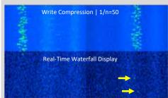
months, waterfall and trace data can become a storage challenge, and requires time-intensive post event analysis, which can be a daunting process. The unique write management feature, in combination with the ability to compress the trace and waterfall data, is a powerful innovation that significantly improves the operators analysis and review capability. Kestrel's spectrum and waterfall compression method
