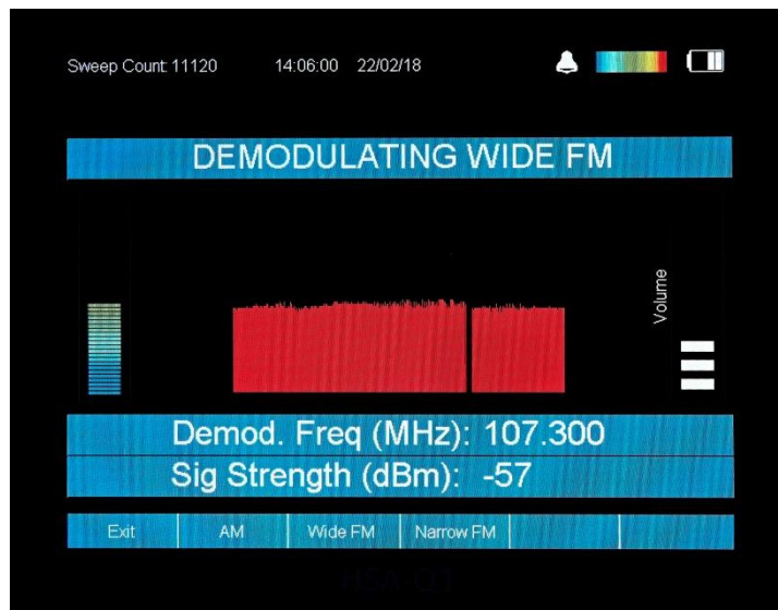
Tune Listen Mode – Signal at 107.3 MHz (-57 dBm signal strength) - Demodulated Audio in Wideband FM
