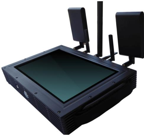
QCC Sentinel is the most advanced portable TSCM system for the detection & location of Wi-Fi 2.4GHz - 5GHz devices / Access Points & for detection & location of / Bluetooth devices (all classes) with full direction finding capabilities. Detect, analyse and locate all Wi-Fi and Bluetooth devices. (Connected and Unconnected)
