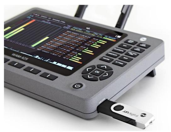
element signal strength meter enabling the precise source of a detected signal to be located with ease. An audible 'Beep' mode allows the user to monitor without looking at the display and a silent Vibrate mode can also be used for particularly sensitive areas.
