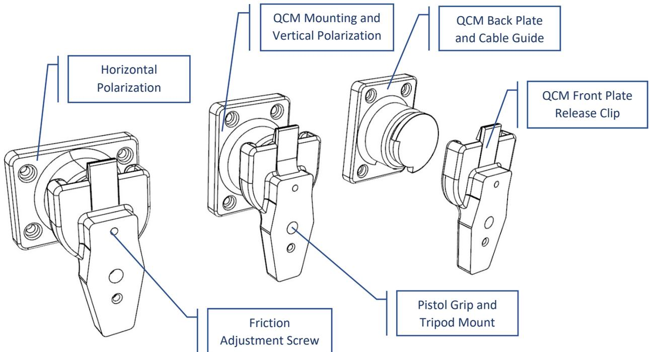
The locking | **QCM Front Plate** | supports the pistol grip and tripod combination (included), and permits the use of any standard tripod configuration (not included) to be utilized for unique deployment or temporary mounting applications.
