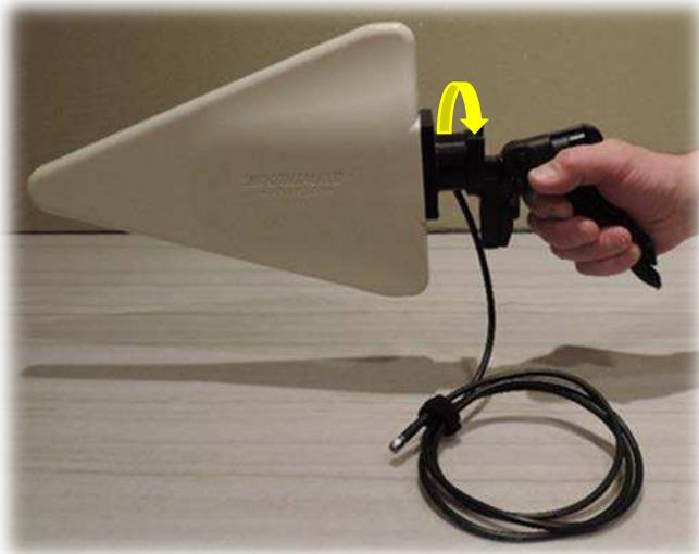
To change the antenna polarization to the horizontal position, the antenna is turned 90 degrees (counter-clockwise) from vertical to achieve horizontal polarization.
