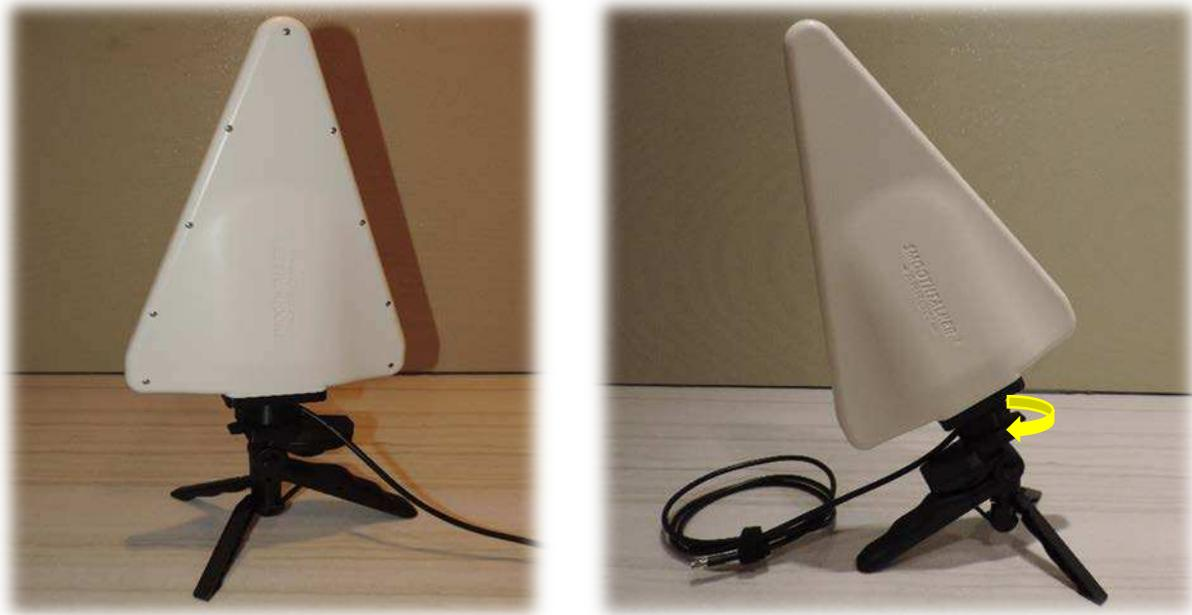
The polarization can be adjusted up to 90-degrees depending on the target area orientation with reference to the antenna Null regions, off each narrow edge of the antenna.
