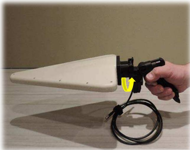
When the antenna is oriented in the horizontal polarization, the antenna rotates 90 degrees (clockwise) back to the vertical polarization position.
