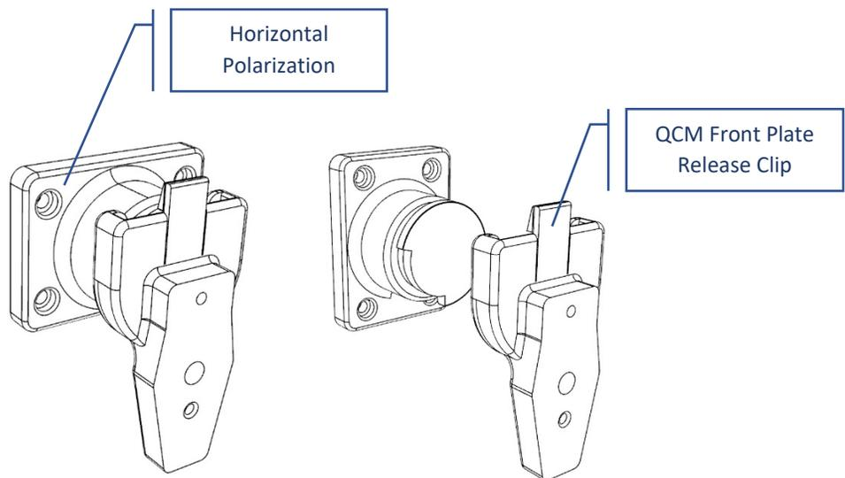
The | **Quick Connect Mechanism (QCM)**™ | is a 90-degree rotatable friction assembly, manufactured with a strong durable material that is light weight, reduces fatigue during deployment, and the compact nature of the Kestrel Log Periodic (KLP)™ antenna kit, is ideal for travel.
