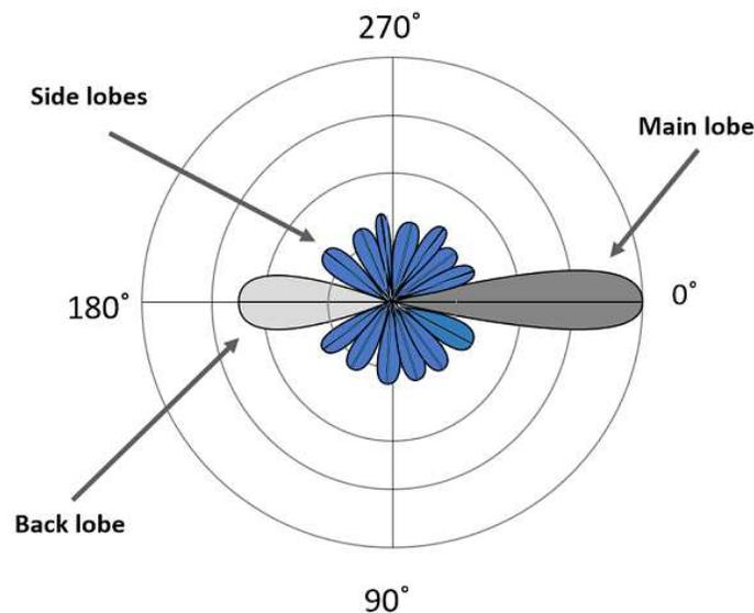
The directional Beam Width of the KLP antenna is approximately 85 degrees when oriented in the vertical position and requires that the technical operator make significant directional shifts when determining direction, based on the Relative Signal Strength Indicator (RSSI).
