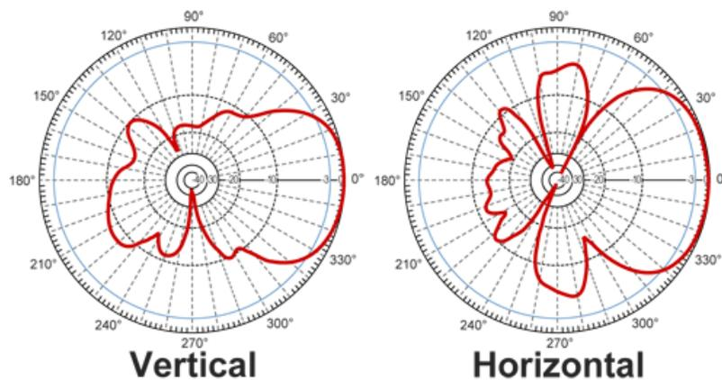
The example LPA plots above, illustrate the differences between the vertical and horizontal antenna polarization patterns and are typical of most Log Periodic Antenna (LPA) designs.
