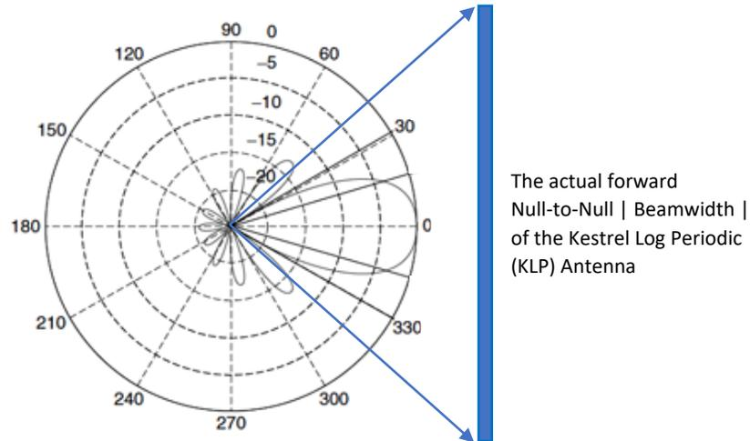
All elements of a Log-Periodic Antenna (LPA) are considered to be “active” in nature, or electrically connected to the antenna feedline, along with all other elements, with each successive element connected in opposite phase.
